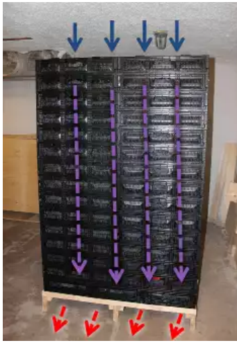
Figure 3. This column vertical airflow system uses RPCs with bottom vents. Cold air (blue arrows) is pulled vertically down from the top of the stack (purple then red arrows) through a specially designed pallet using a high-capacity fan located at the base (not shown). RPCs work well because they have fully vented bottoms, cross-stack on alternating layers, fit perfectly on a standard pallet and fit so tightly against each other that there are no spots where cold air can short-circuit. All four vertical sides of the stack must be covered with tarps (not shown) to compel cold air to travel vertically. (Photo courtesy of Dr. Bernard Goyette, Vineland Research and Innovation Centre, Vineland)
